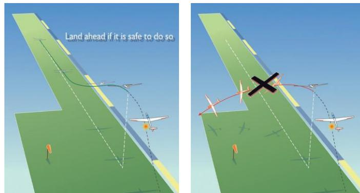
*Sink* is one such hazard, often associated with strong winds and wave. A glider making a 360° turn in still air at a bank angle of 35° and 50 knots typically descends by only 70 feet. But with 15ft/second sink the height loss in a 360° turn is over 400 feet. If the launch failure was at 300 feet the glider would crash before completing a 360° turn.
